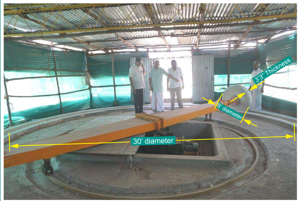
Dr. Arun Menon - IIT Consultant, Mr. V S Jayabal - Donor and Mr. Kumragurubaran - Sthapathi discussing a Lime-Mortar mixer arrangement
